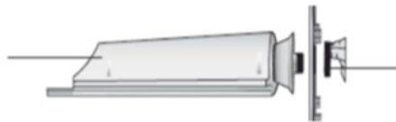
1. Body of the device 2. Base 3. Securing nut
