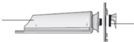
1. Body of the device 2. Base 3. Securing nut
