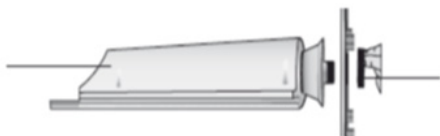
1. Body of the device 2. Base 3. Securing nut
